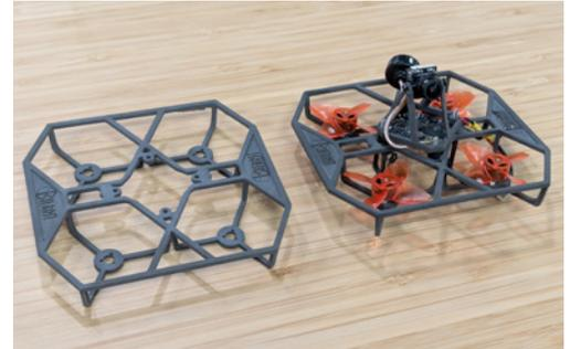
A camera drone frame (left) 3D printed with SAF technology and the completed assembly (right).
