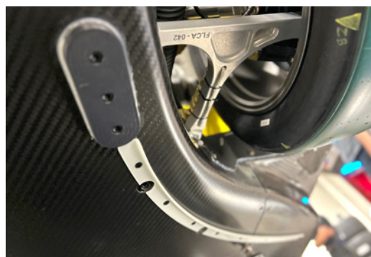
A strake (white) installed on the underside of the race car.
