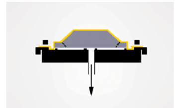
Figure 14: Vacuum is drawn to remove air from between the tool and sheet.
