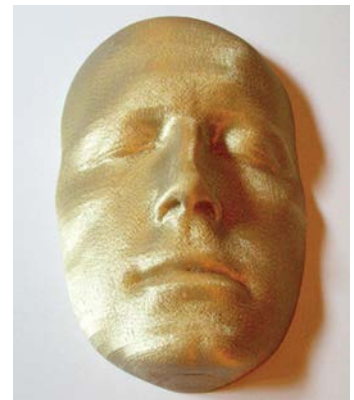
Figure 6: FDM tool, made in PPSF/PPSU, has formed more than 500 parts with no sign of wear
