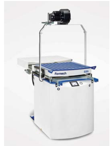
Figure 8: The Formech 686 is an example of a semi-automatic thermoforming system. A system such as this works well with FDM-produced tooling.
