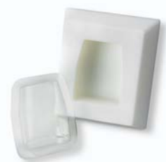
Packaging thermoformed using an FDM mold.
