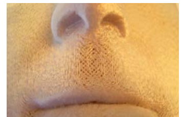
Figure 7: Close up of the tool in figure 6 shows the porosity that results from modified build parameters.
