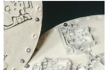
Figure 8: After the metal has cooled, separate the mold to expose the castings.
