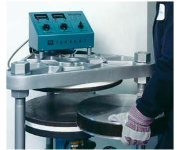
Figure 4: The mold is loaded into a vulcanizer that cures the rubber.
