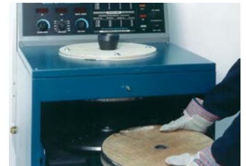
Figure 6: The mold is loaded into the spin casting machine.
