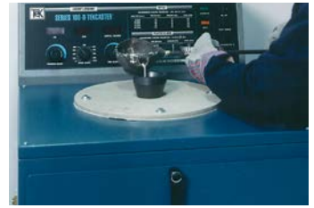
Figure 7: While spinning, molten metal is poured into the mold.
