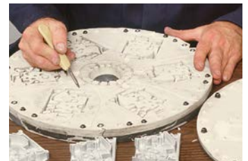
Figure 5: Gates, runners and vents are cut into the rubber mold with a sharp knife or scalpel.
