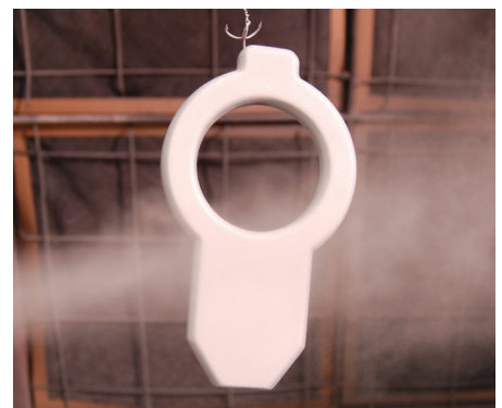
Figure 29: Using good-quality paint, apply several thin coats.
