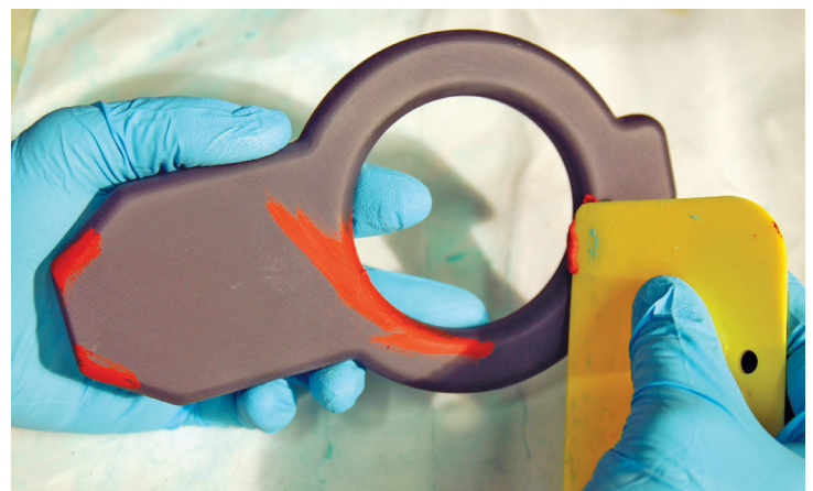
Figure 26: If surface imperfections remain, fill them with a glazing putty (or similar) that feathers nicely.
