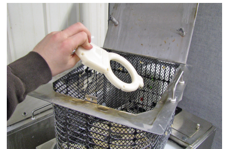
Figure 13: Remove part from tank when no support material remains.
