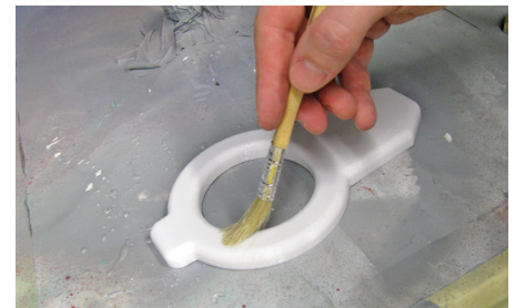
Figure 16: Solvents may be brushed on surface of ABS and PC parts to smooth them.
