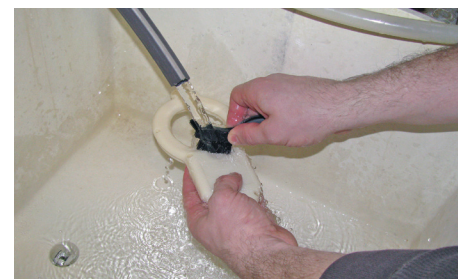
Figure 14: Thoroughly wash part to remove any residual solution.
