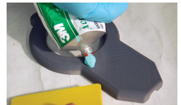
Figure 21: Apply a small amount of spot putty or body filler.
