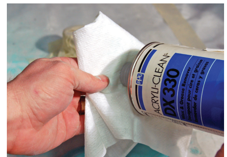
Figure 18: Wipe all surfaces with a degreaser to ensure good adhesion.
