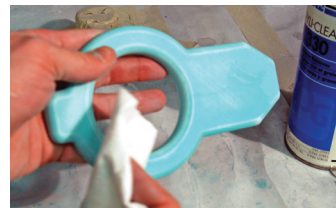
Figure 24: Between each step, clean and degrease surfaces to have good adhesion of filler, primer and paint.
