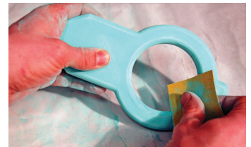
Figure 23: Allow filler to dry and then sand all surfaces to desired smoothness.
