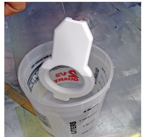
Figure 17: Alternatively, parts may be dipped in solvent.
