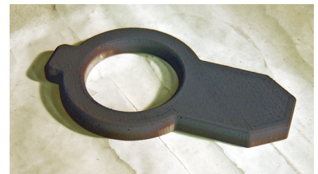
Figure 19: A coat of primer will highlight areas that need sanding and filling.
