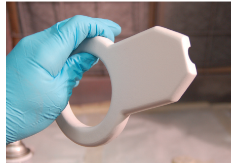
Figure 31 : Between coats, lightly sand for adhesion and inspect for any surfaces mars.
