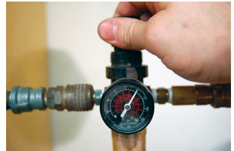
Figure 32: For textured finishes, when using a spray gun, adjust pressure and flow rate.
