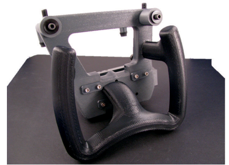
Figure 9: FDM badge alignment fixture is lightweight because of its plastic construction and use of sparse fill build styles.
