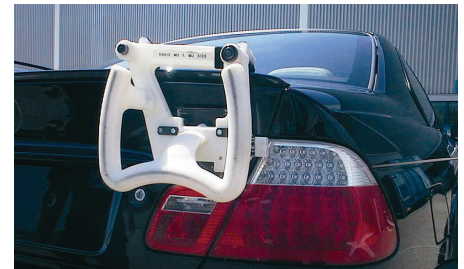
Figure 8: Redesigned FDM fixture consolidates most components and is optimized for ergonomics.
