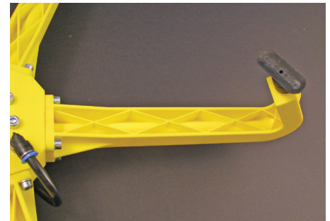
Figure 11: Each arm for a “robotic gripper” has integrated vacuum channels and generous ribbing.
