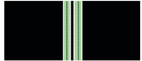
Figure 50: Defaults may produce voids in thin walls when rasters cannot fill between contours.
