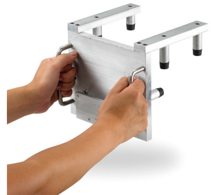
Figure 7: Machined metal fixture made of over two dozen parts.
