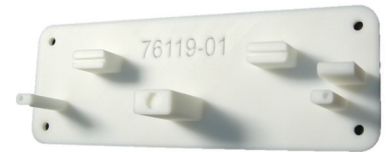
Figure 36: Select thinner slices for small features, smooth surfaces and dense fills.
