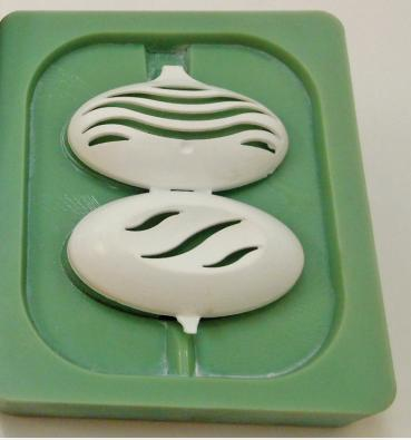
Using 3D Printing, Unilever can produce prototypes in the final material for functional and consumer testing 40 percent faster than before.
