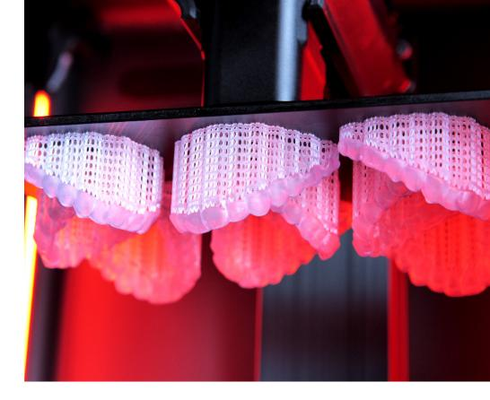
technology from Stratasys allows for the mass production of functional end-use parts. A programmable, carefully orchestrated print process maximizes strength and production speed, and highperformance photopolymer materials result in optimal strength and precision. The Origin<sup>®</sup> One Dental 3D printer incorporates this technology to help labs scale up production of dental models, splints, and surgical guides.
