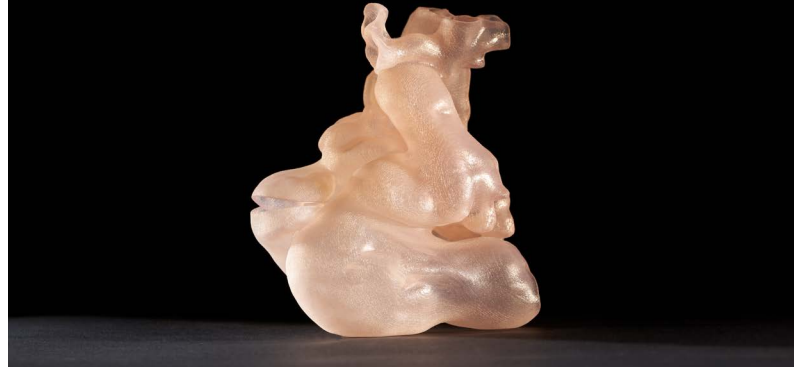
Figure 2a: Functional model created using a custom Agilus30™ and Vero™ White multimaterial blend.
