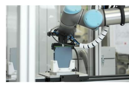
For the robot grippers, additive manufacturing enables the compact design, and applications such as complex vacuum channels in the basic body can be realized.
