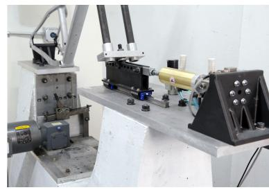
Black 3D printed carbon fiber-filled nylon 12 holding fixtures anchor a bike frame during fatigue testing.
