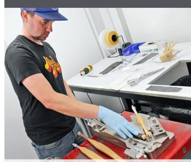
Test fitting a 3D printed ULTEM™ 1010 resin mandrel in the composite lay-up tool used to make the carbon fiber bike frame.
