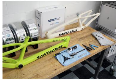
Design concept bike frames 3D printed using ASA material.
