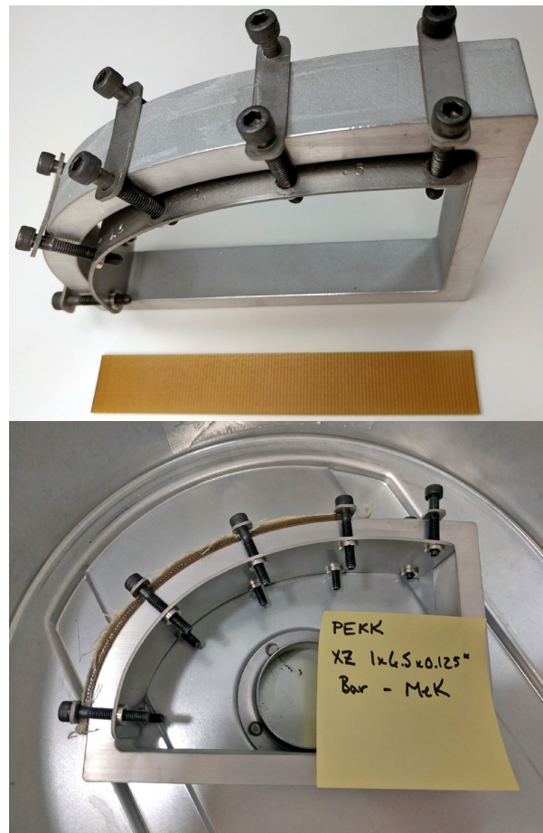
Figure 2: Variable Strain Fixture - shows the extent of deformation under various strains with chemical exposure. Some samples broke above 1% strain with certain chemicals.
