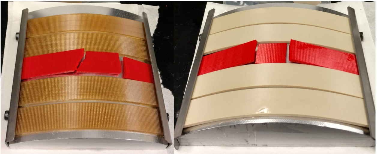
Figure 7: Non-annealed (left) and annealed (right) specimens after exposure to Skydrol (orange = ULTEM 9085 resin)
