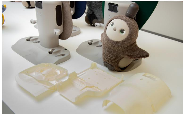
Not only LOVOT's main unit, but also its larger charger is prototyped by a 3D printer.
