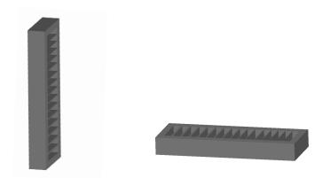
**Figure 1:** Via the left side orientation, the walls are horizontal with relation to the surface of the build where the build top is located at the uppermost surface; therefore this orientation will be referred to as the horizontal orientation. Via the orientation shown on the right, the internal walls are vertical in relation to the surface of the build therefore this orientation will be referred to as the vertical orientation.
