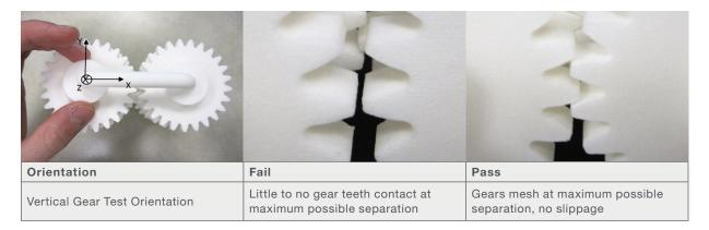
Table 7: Pass/ fail criterion for gears manufactured in LS.
