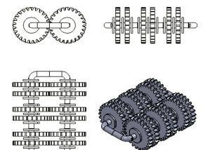
**Figure 6:** This gear was designed to test how much the center distance can be varled before fusing occurs and or before the gears fail to mesh during rotations. The three gear pieces test separate sizes with 15-20 teeth. Gear pairs run the length of the design. The center distance is gradually increased by 0.5 mm.
