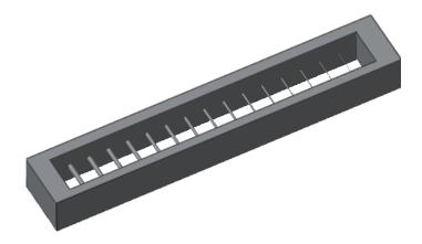
Figure 8: The pins within this design have varied diameters beginning as small as 0.2 mm and ending at the largest 3 mm in diameter.
