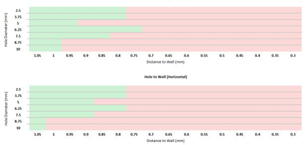
**Table 3:** Pass/fail matrices for hole diameters and distance from other features (in this case, the edge or wall of the part).
