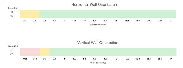
**Table 1:** Red designates a complete failure to build, yellow designates a passing build with significant inaccuracies, and green represents a complete build for each wall thickness.
