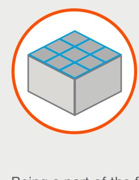
Sparse fill means less material built into the part, so the weight of the final part is significantly reduced. The reduction in material and faster print time contributes to a cheaper overall part.
