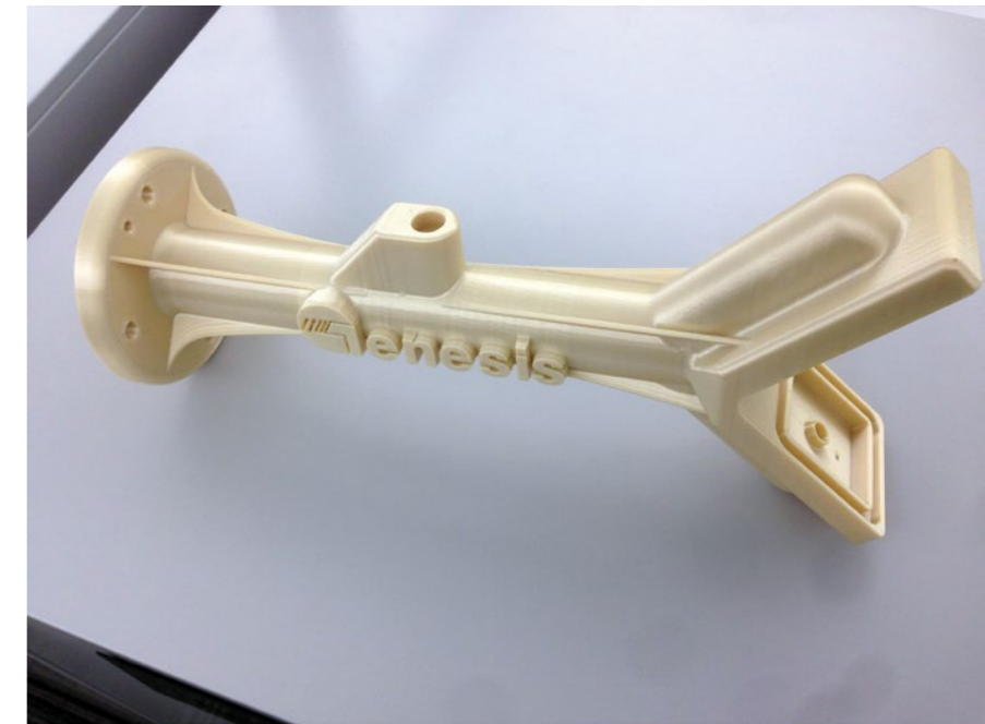
A lightweight FDM end effector designed by Genesis Systems Group incorporating integral vacuum channels.
