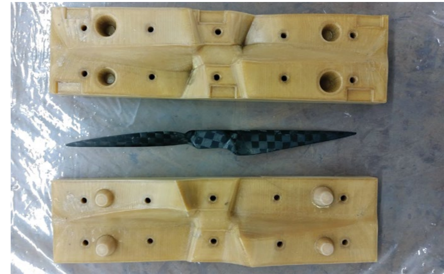
ULTEM 1010 resin forming tool used to create composite UAV propeller blades.
