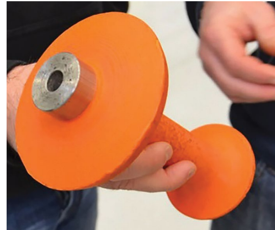
A lightweight but durable punching tool produced on a Fortus 3D Production System.
