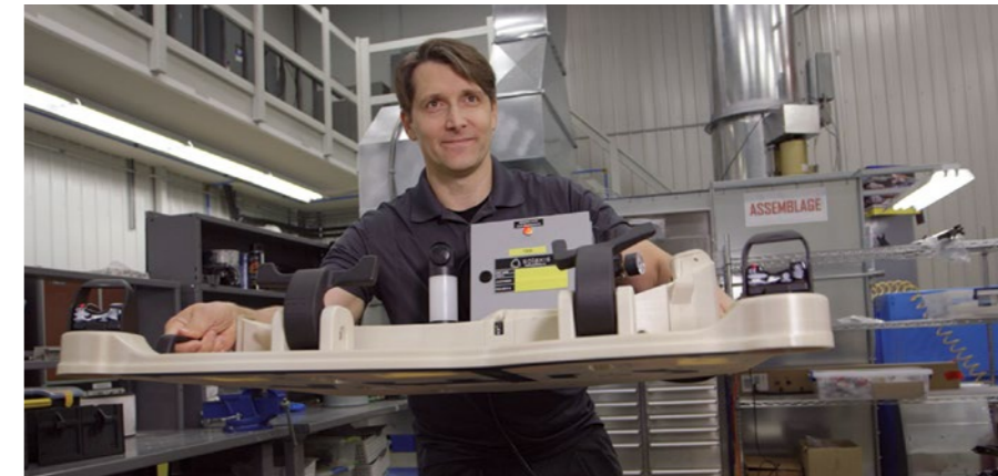
This assembly jig made with Fortus FDM materials is only a fraction of the weight it would exhibit if made from metal.
