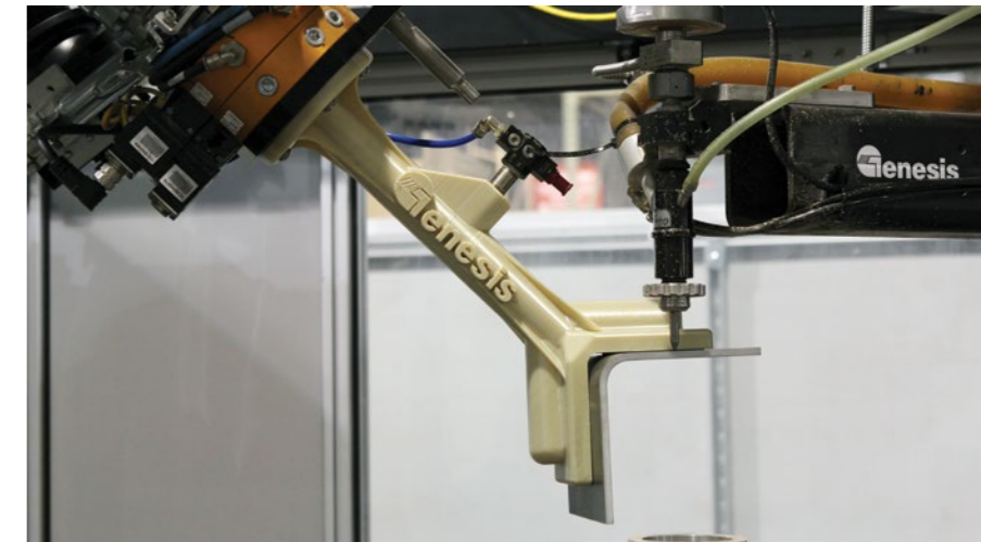
The end effector in use in a waterjet cutting operation.
