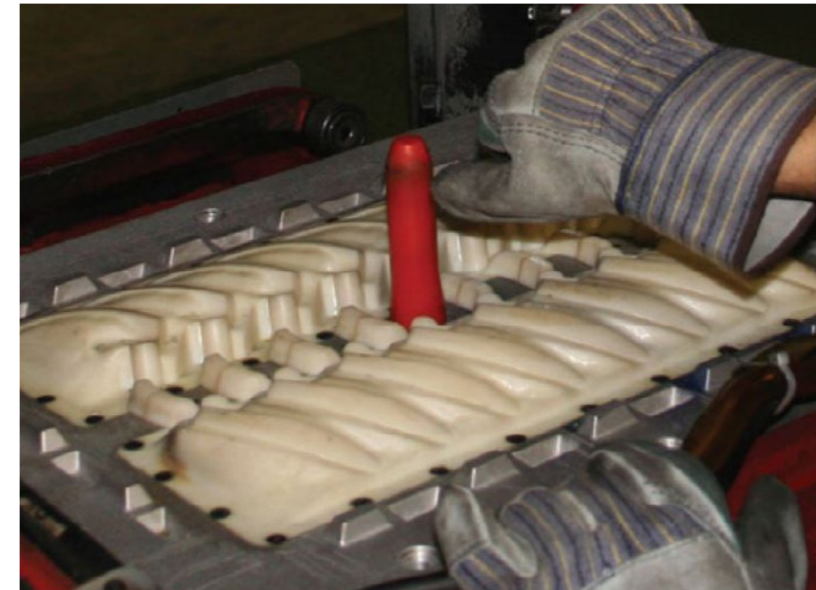
Matchplate with FDM insert in molding machine.
