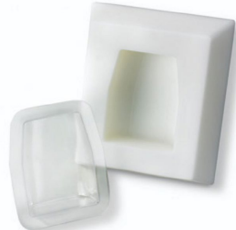
Thermoformed packaging cover and FDM mold.
