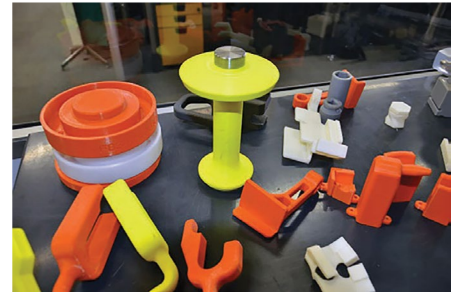
Volvo Trucks used FDM technology to dramatically reduce the time required to produce jigs, tools and assembly aids.
