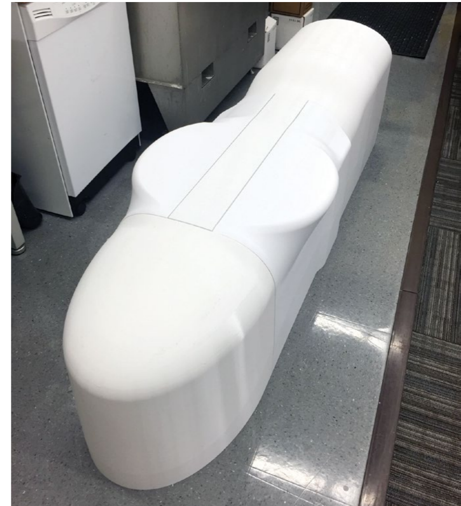
The belly pod forming tool assembled from several sections produced on a Fortus 900mc 3D Printer.
