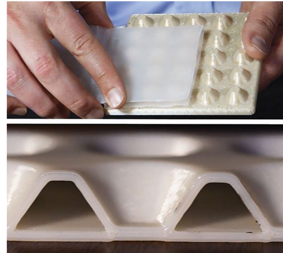
The FDM tool (top) was used to proof and then produce the dimpled design of the lightweight, twin-sheet trunk plate.
