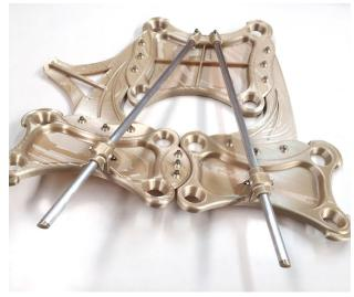
Indaero redesigned and 3D printed a tool nine kilos lighter than the traditionally manufactured tool.
