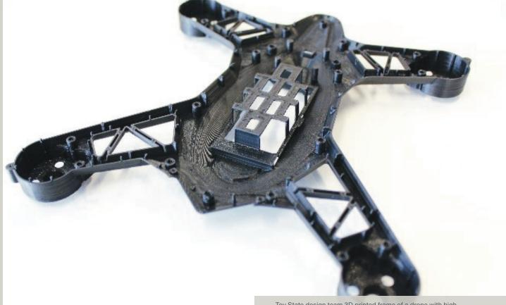
Toy State design team 3D printed frame of a drone with high precision and strength using PC- ABS material.
