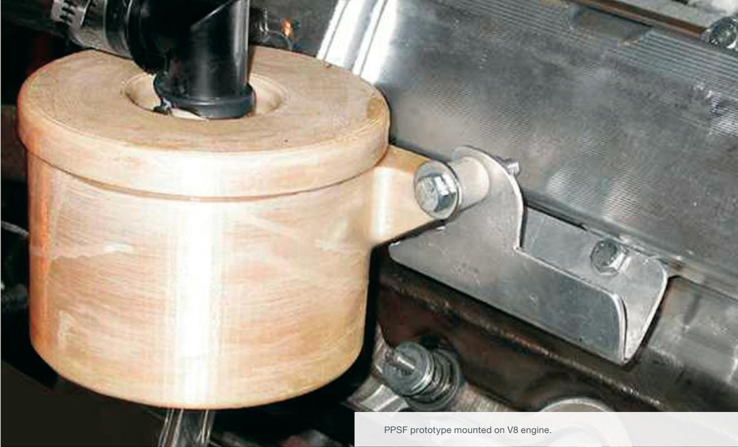
PPSF prototype mounted on V8 engine.
