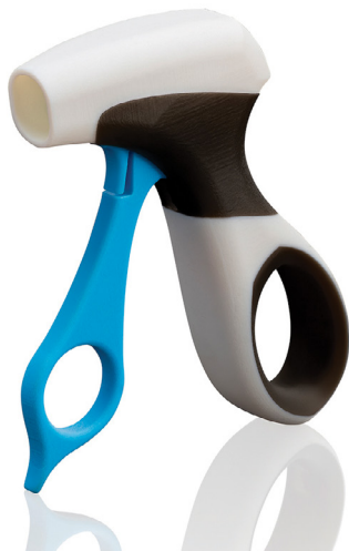
Figure 7. Digital ABS Plus features heavily in this design verification prototype for medical devices. This surgical prototype also features Agilus30 overmolding in black for superior grip and a 3D printed color handle, printed separately. Digital ABS Plus has heightened impact strength from Digital ABS, leading to improved functional performance.
