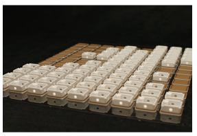
Optimize the orientation and pack of a build for maximum throughput, like these polycarbonate parts.
