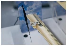
Aurora made this wing entirely of 3D printed components and 3D printed electronics.
