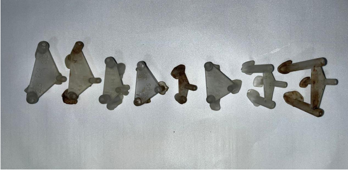
3D printed models of patient-specific jigs were printed using the Stratasys J5 MediJet 3D printer in Med-610 biocompatible material.
